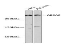
Western blot analysis of extracts of various cell lines, using ABCA2 Polyclonal Antibody at 1:1000 dilution.<br/>
