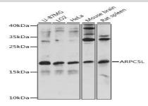
Western blot analysis of extracts of various cell lines, using ARPC5L antibody.
