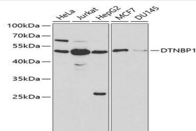
Western blot analysis of extracts of various cell lines, using DTNBP1 antibody at 1:1000 dilution. Secondary antibody: HRP Goat Anti-Rabbit IgG at 1:10000 dilution. Lysates/proteins: 25ug per lane. Blocking buffer: 3% nonfat dry milk in TBST.
