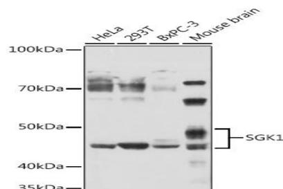
Western blot analysis of extracts of various cell lines, using SGK1 antibody at 1:1000 dilution. Secondary antibody: HRP Goat Anti-Rabbit IgG at 1:10000 dilution. Lysates/proteins: 25ug per lane. Blocking buffer: 3% nonfat dry milk in TBST. Detection: ECL Basic Kit. Exposure time: 90s.
