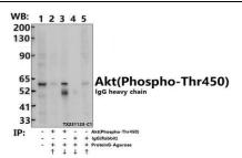
Immunoprecipitation of 3T3-L1 cell lysates using AKT (phospho-T450) pAb (Sepharose Bead Conjugate)#BD0048 (lane 2 and lane 3) and Nonspecific IgG Control (Sepharose Bead Conjugate)#BD0048 (lane 4 and lane 5) .Lane 1 is 30% input. The western blot was probed using AKT (phospho-T450) pAb.
