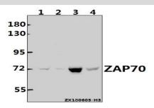
Western blot (WB) analysis of ZAP70 (T286) at 1:500 dilution Lane1:THP-1 whole cell lysate(40ug) Lane2:Myla2059 whole cell lysate(40ug) Lane3:HuT78 whole cell lysate(40ug) Lane4:The Thymus tissue lysate of Rat(40ug)
